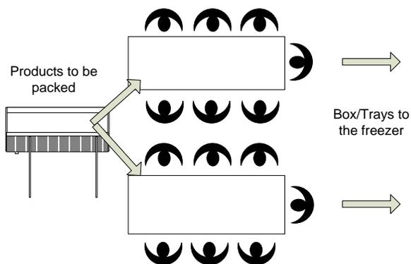
Figure 10. Alternative distribution of the wrapping workstation
