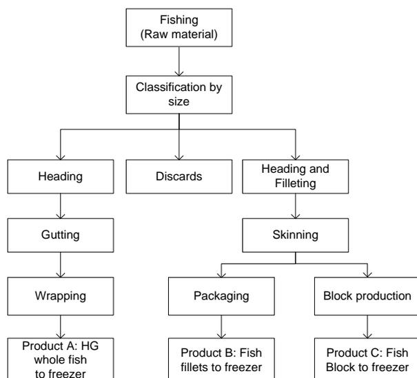
Figure 1. Flow diagram of the factory ship process
