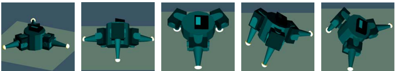
Figure 3: Sequence of five consecutive actions for the tripod robot while the models are random. The position of the legs will change continuously until the models become correct and the desired configuration (three legs up) is achieved.
