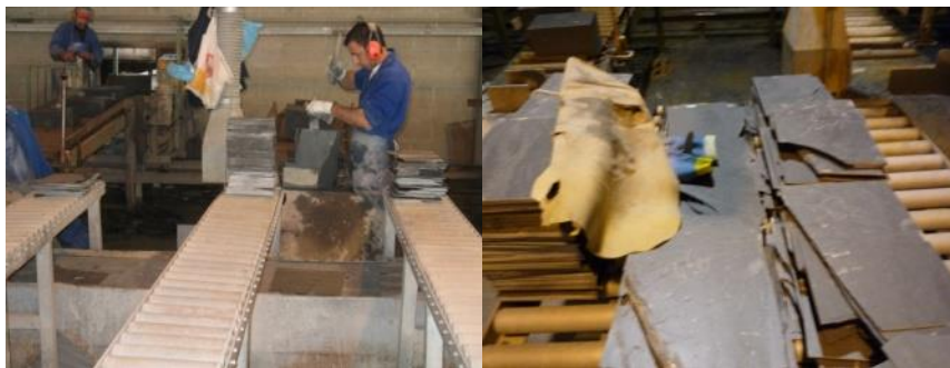
Fig. 3. A Splitter (left) and the Resulting Output: The Target Formats (regular lots in the left) and Secondary Less Quality Output Formats (the two series in the right).
