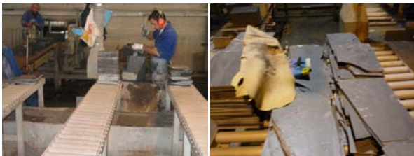
Figure 3: A Splitter (left) and the Resulting Output: The Target Formats (regular lots in the left) and Secondary Less Quality Output Formats (the two series in the right).
